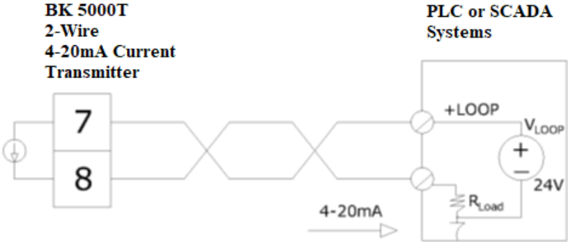
Figure 7: BK5000-T 4-20 mA Current Transmitter Wiring Diagram
