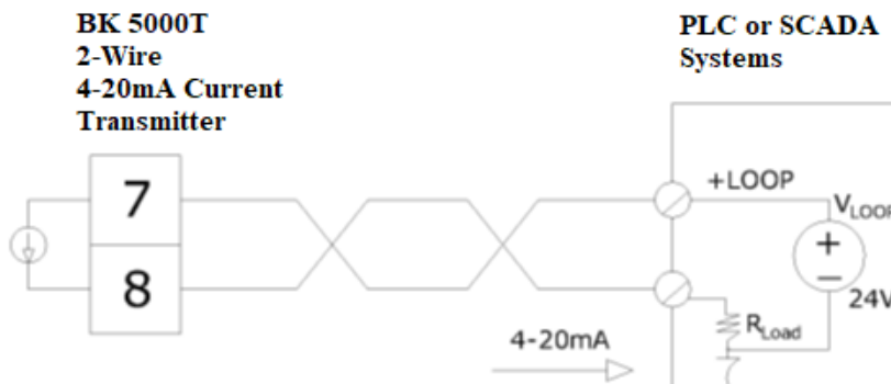
Figure 7: BK5000-T 4-20 mA Current Transmitter Wiring Diagram
