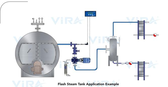
To achieve maximum flash steam, the maximum amount of condensate is required. For this reason, the capacity of the steam traps should be carefully selected taking into account the counter-pressure capacity. Also, in systems with temperature control valves, it should be taken into account that the pressure will drop as soon as the valve is closed.
